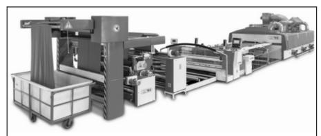
The Motex 15000 also achieves consistent and reproducible results across the length and width of the fabric, even with larger overfeed adjustment range up to 80%. The Stenter enables the processor to achieve even drying and heat setting at higher evaporation rates with optimum energy utilisation, which translates into lower operating cost per metre of fabric.
