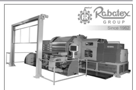
The Rabatex high speed Sample Warping Machine model RI 6001 is primarily for production of samples and short production warp at very high production rate.
